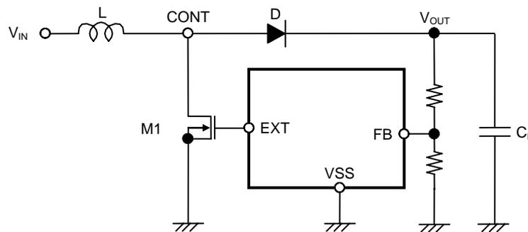
**Figure 10 Step-up Switching Regulator Circuit for Basic Equations**
