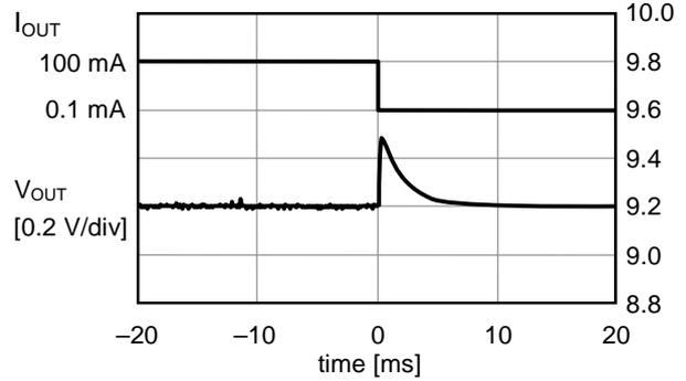
(5)  $f_{OSC} = 286\text{ kHz}$ ,  $I_{OUT} = 0.1\text{ mA} \rightarrow 100\text{ mA}$
