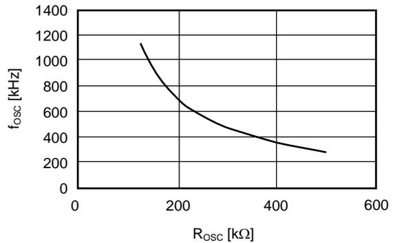
**Figure 12 R<sub>osc</sub> vs. f<sub>osc</sub>**
