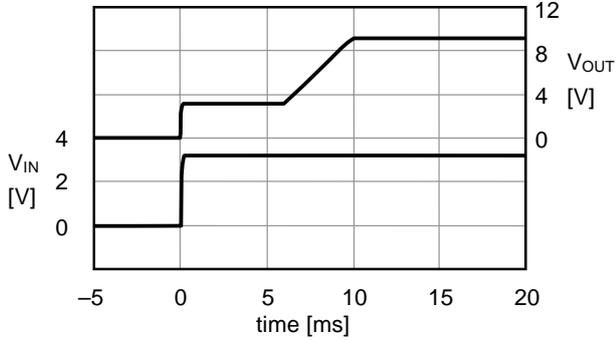
(2)  $f_{OSC} = 1133\text{ kHz}$ ,  $I_{OUT} = 100\text{ mA}$ ,  $t_{SS} = 10\text{ ms}$
