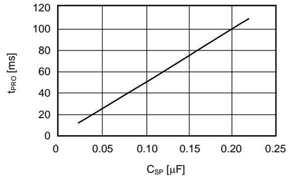
**Figure 14** C<sub>SP</sub> vs. t<sub>PRO</sub>
