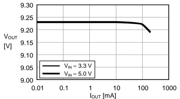
(3)  $f_{OSC} = 286\text{ kHz}$ ,  $MaxDuty = 77\%$  ( $R_{OSC} = 510\text{ k}\Omega$ ,  $R_{Duty} = 750\text{ k}\Omega$ )
