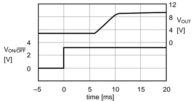
**4. 3 Load fluctuations ( $V_{OUT} = 9.2\text{ V}$ ,  $V_{IN} = 3.3\text{ V}$ ,  $T_a = 25^\circ\text{C}$ ,  $R_Z = 200\text{ k}\Omega$ ,  $C_Z = 0.01\text{ }\mu\text{F}$ )**
