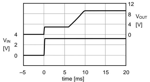
**4. 2 Responses of shutdown pin ( $V_{OUT} = 9.2\text{ V}$ ,  $V_{ON/OFF} = 0\text{ V} \rightarrow 3.3\text{ V}$ )**
